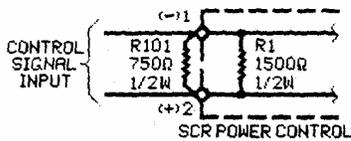
Fig A. Impedance = 500 ohms
