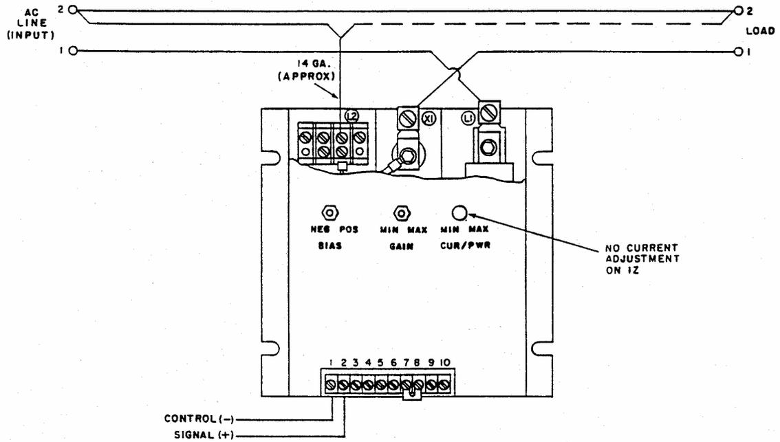
Figure 2-1. Typical 1Z Line and Load Connections
