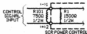
Fig B. Impedance = 1500 ohms
